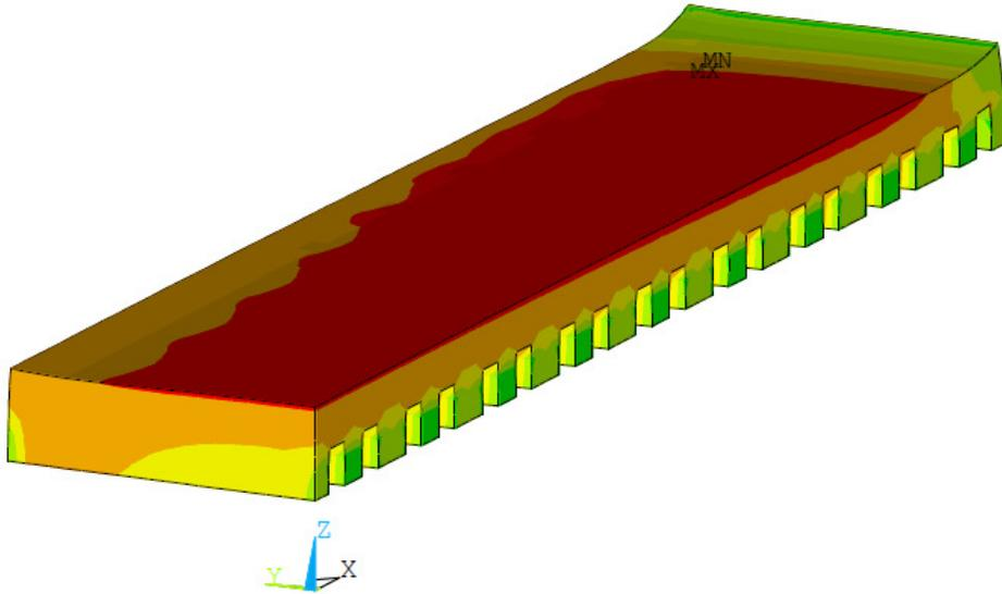
Figure 7: Longitudinal stress component in the cathode panel after 24 of cooling from the 3D quarter cathode cell model
