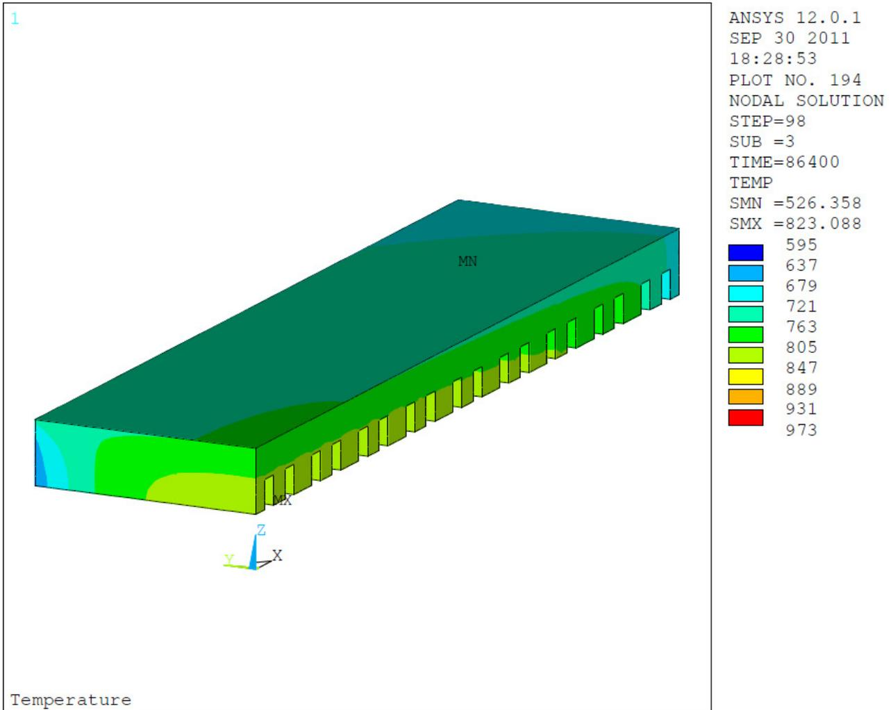
Figure 4: Temperature of the cathode panel after 24 hours of cooling from the 3D quarter cell model
