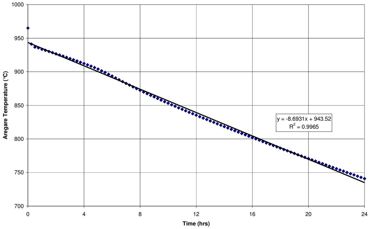
Figure 2: Average metal pad cooling rate from the quarter cell model
