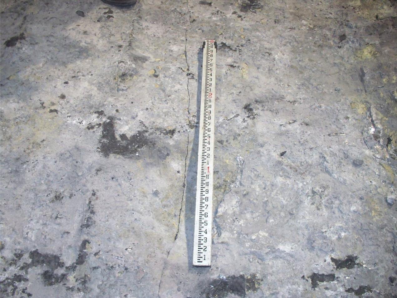
Figure 1: Transverse cathode cooling crack
