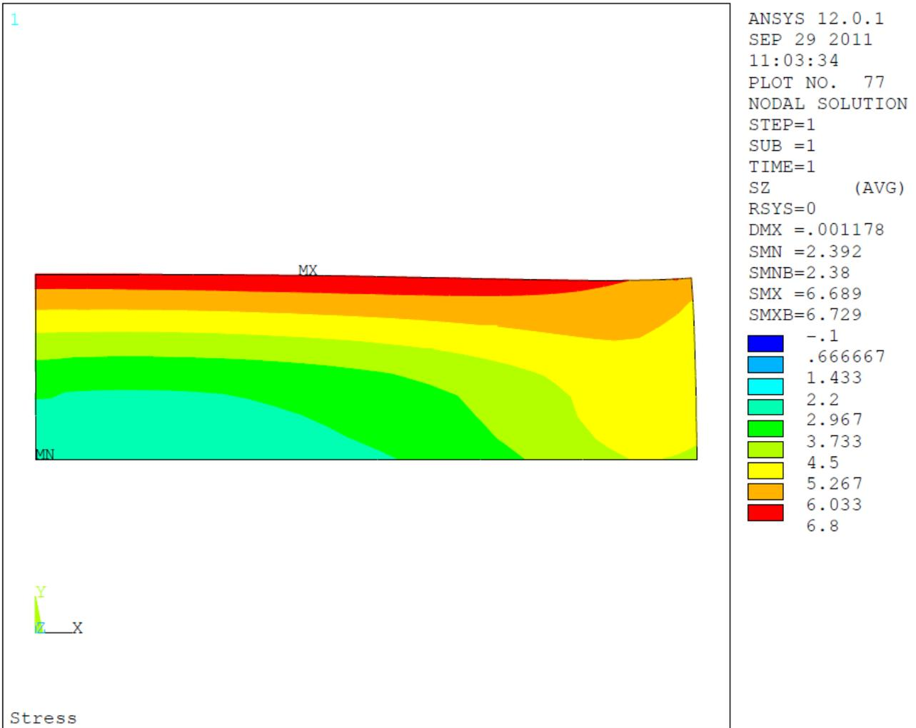
Figure 6: Longitudinal stress component in the cathode block after 24 of cooling from the 2D model
