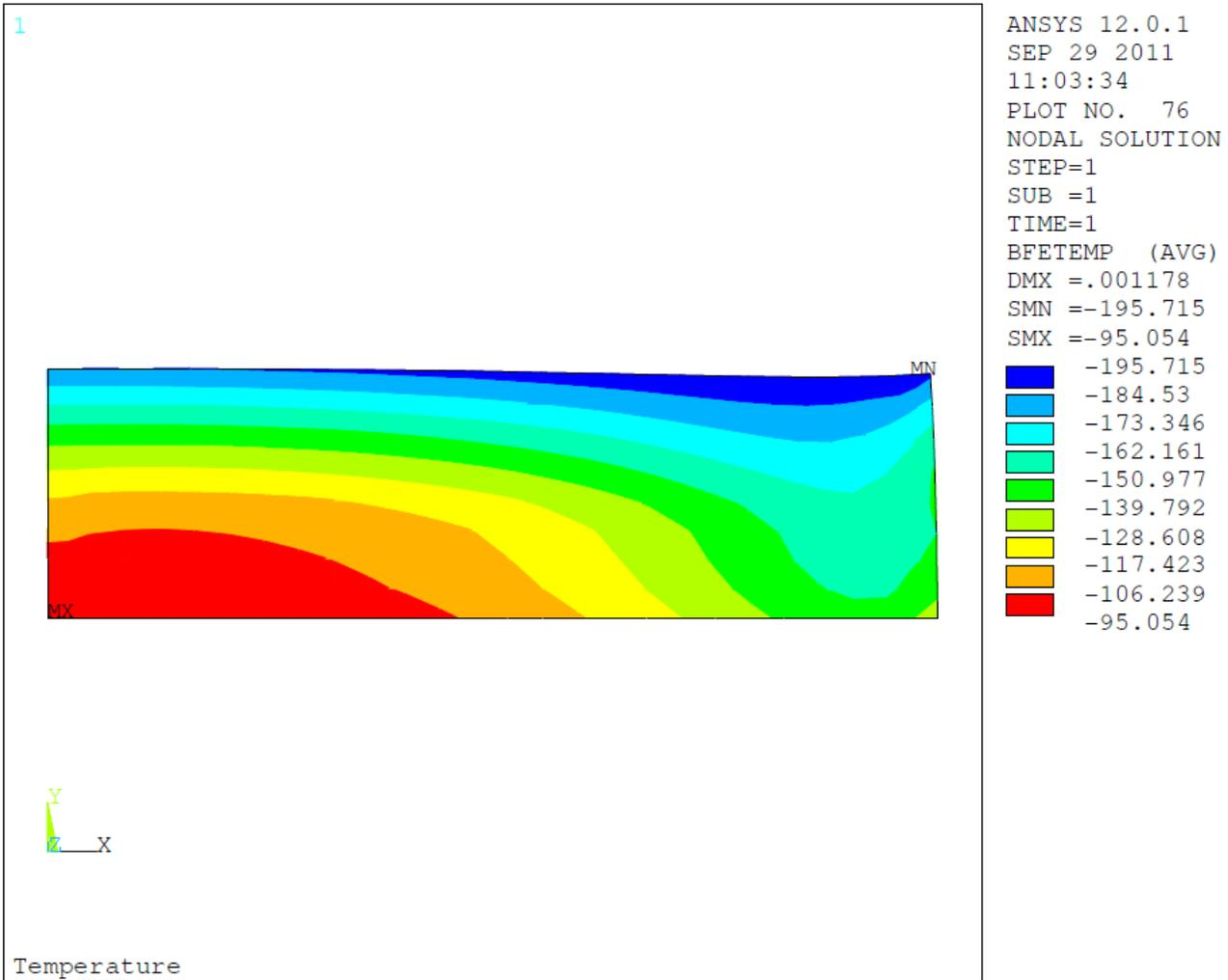
Figure 5: Relative thermal gradient in the cathode block after 24 hours of cooling from the 2D model
